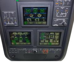
(above) Korry's world-first utility control system with integrated touchscreen controls for the Gulfstream G500/G600/G700 aircraft
