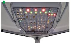
Integrated Switch Panels Korry Integrated Switch Panels (right) are available in a number of formats or can be developed to specific requirements.
